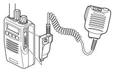
2 Secure the connector in place using the attached screw.
