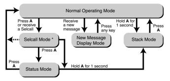
\* Depending on how your dealer programmed the transceiver, Selcall Mode may be skipped or the transceiver may exit Selcall Mode automatically (as shown by the dash arrow).
