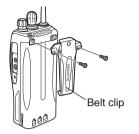
If necessary, attach the belt clip using the two supplied M3 x 8 mm screws.
