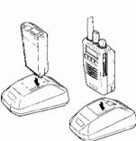
**Note:** When charging a transceiver with a Li-ion battery pack, the safety catch of the battery pack may stick out past the battery. When inserting the transceiver with the battery pack into the charger, the safety catch will touch the metal contacts of the charger and the charger LED will momentarily light red. Be sure to push the transceiver fully into the battery pack slot so the safety catch no longer touches the charger terminals. Once in place, the battery pack will begin charging.
