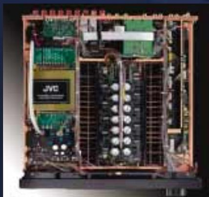
a thick (1/16 inch), isolated base. This sophisticated design prevents digital and video noise from mixing with the delicate audio signals. Result: better sound quality.
