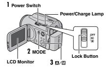
Set the appropriate operation mode according to your preference using the power and **MODE** switches and  $> (\square/\square)$  button.
