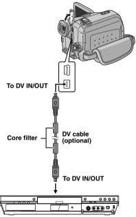
Video unit equipped with DV connector
