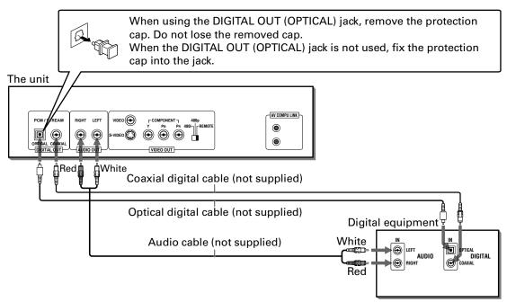
• For digital connection, connect the unit's DIGITAL OUT (OPTICAL or COAXIAL) to the digital input of digital audio device using an optical or a coaxal digital cable.
