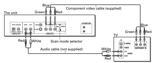
• Connect "Y" to "Y", "PB" to "PB"(CB), "PR" to "PR"(CR) correctly.
