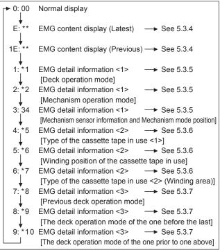
EMG display of 7 FDP display model Fig.5-3b
