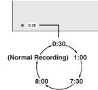
When the unit reaches the specified time, it will be turned off automatically.
