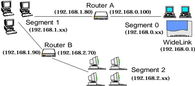
Figure 23: Routing Example
