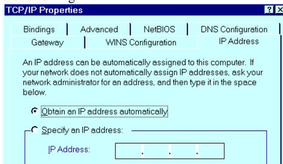
**Figure 9: TCP/IP Properties - DHCP**
