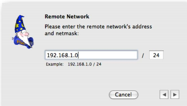
Enter the remote network address and netmask (please note that the netmask needs to be entered in **CIDR** format). This has to match with the settings of the FVS328.
