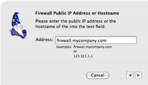
Enter the public IP address or hostname of your Netgear FVS328 router. In case your ISP assigned you a dynamic IP address, you should register with a dynamic IP DNS service (like <http://www.dyndns.org>).
