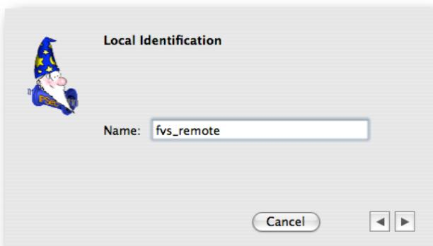
Enter the FVS328's local identification (which is **fvs\_remote** by default if you used the FVS328's wizard).
