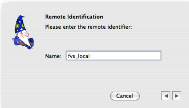
Enter the FVS328's remote identification (which is **fvs\_local** by default if you used the FVS328's wizard).
