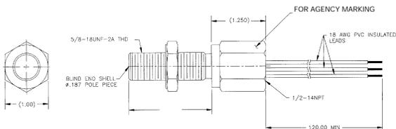
SENSORS WITH 5/8-18 UNF-2A MOUNTING THREAD,
