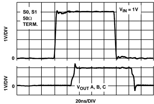
FIGURE 22. CHANNEL TO CHANNEL TRANSIENT RESPONSE  $V_{IN} = 1V$
