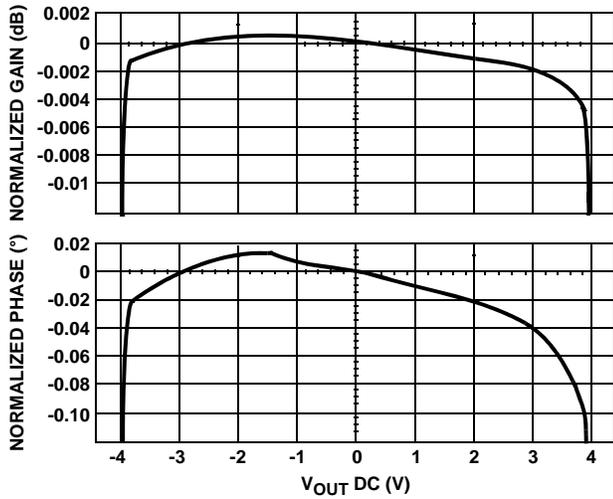
FIGURE 13. DIFFERENTIAL GAIN AND PHASE;
