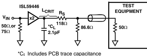
FIGURE 29D. 150Ω TEST CIRCUIT WITH 50Ω LOAD
