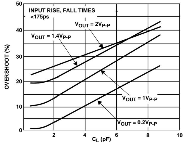
FIGURE 20. PULSE OVERSHOOT vs  $V_{OUT}$ ,  $C_L$ ;  $R_L = 150\Omega$
