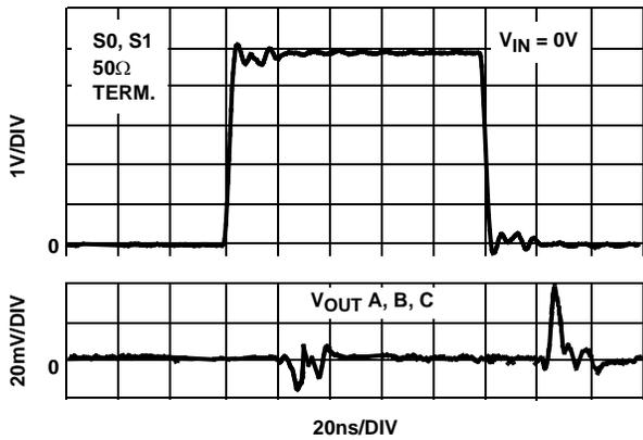
FIGURE 21. CHANNEL TO CHANNEL SWITCHING GLITCH  $V_{IN} = 0V$
