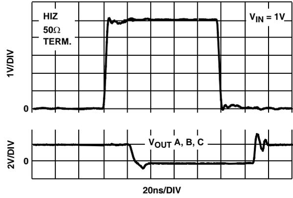
FIGURE 26. HIZ TRANSIENT RESPONSE  $V_{IN} = 1V$
