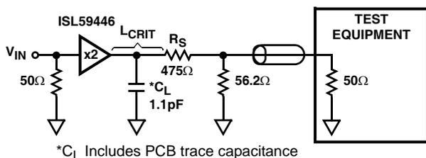
FIGURE 29C. 500Ω TEST CIRCUIT WITH 50Ω LOAD
