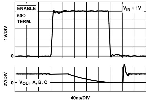
FIGURE 24. ENABLE TRANSIENT RESPONSE  $V_{IN} = 1V$
