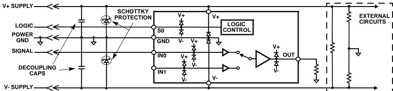
FIGURE 30. SCHOTTKY PROTECTION CIRCUIT
