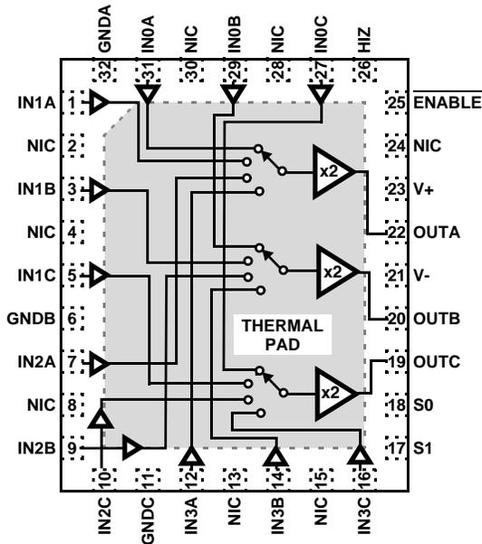
THERMAL PAD INTERNALLY CONNECTED TO V-. PAD MUST BE TIED TO V-
