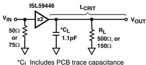
FIGURE 29A. TEST CIRCUIT WITH OPTIMAL OUTPUT LOAD
