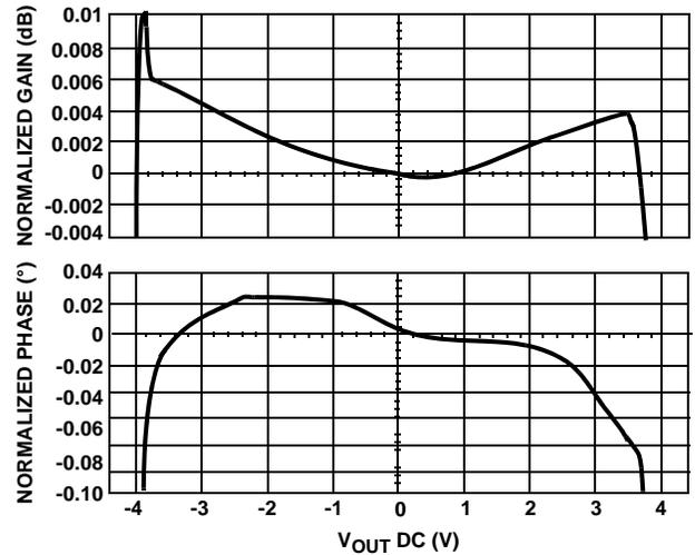
FIGURE 14. DIFFERENTIAL GAIN AND PHASE;
