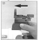
3) Unfasten the alignment clamp by turning counter-clockwise and set the finder body roughly in parallel with the telescope tube. Then, fasten the alignment clamp by turning clockwise.
