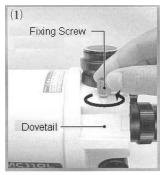
2) Attach the XY Dot Finder to the telescope as shown in the figure 2, tighten the finder bracket fixing screw securely (The mounting block is made of plastic and over tightening the fixing screw may cause damage.).
