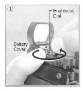
2) Push down the rim of the battery to squeeze out the battery from the battery container. Remove it and replace with a fresh battery.
