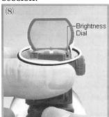
Do not force the brightness dial. This may damage your adjustments for alignment.
