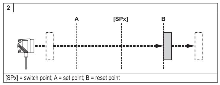
If the output function [Hnc] has been selected, the set and reset points are reversed. The output switches off when the object approaches. When the object is removed again, the output switches.
