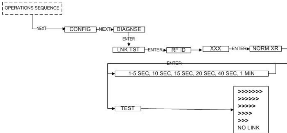
Figure 3-4: Transmitter Link Test
