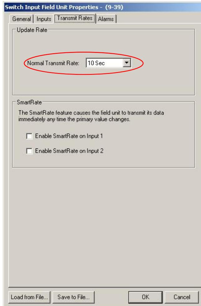
Figure 6-2: Transmit Rates Tab
