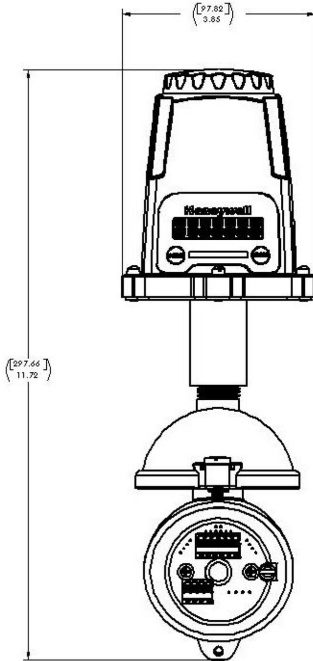
Figure 9-1: Dimensioned Mechanical Drawing
