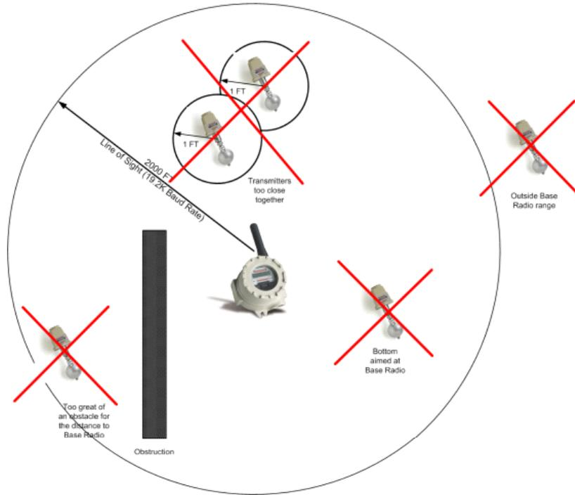
Figure 3-1: Examples of Incorrect Transmitter Positioning
