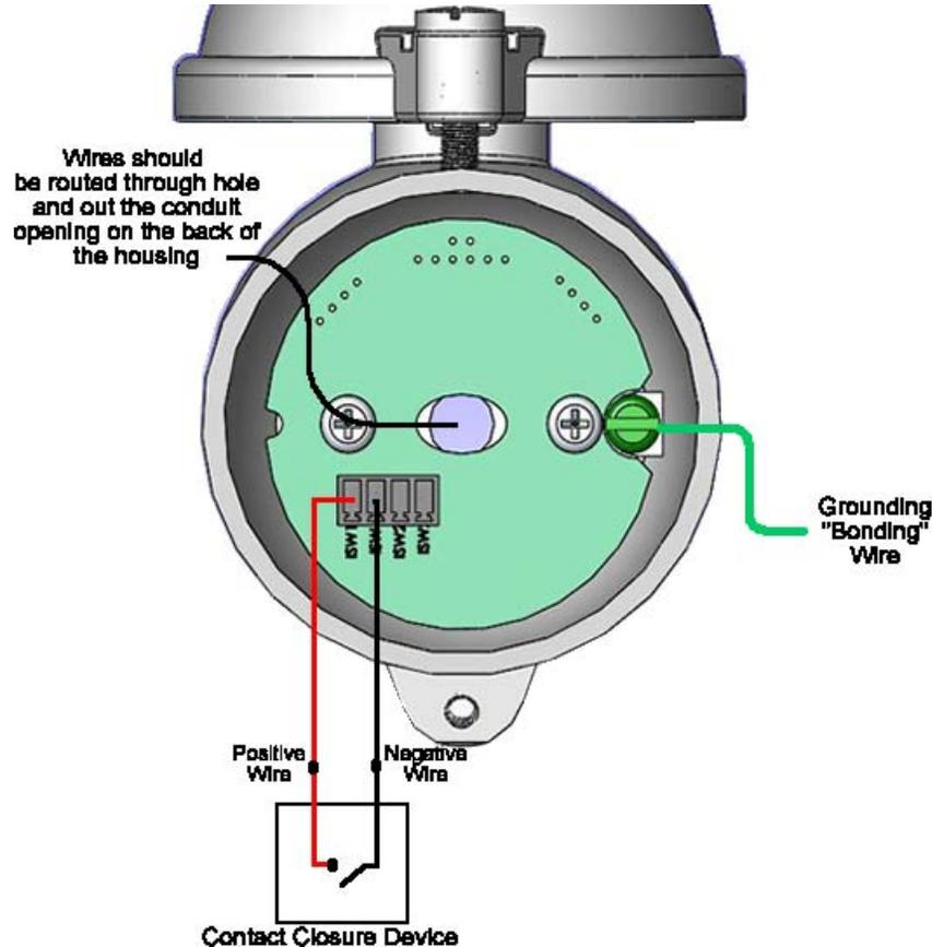
Figure 2-1: Input Switch Wiring
