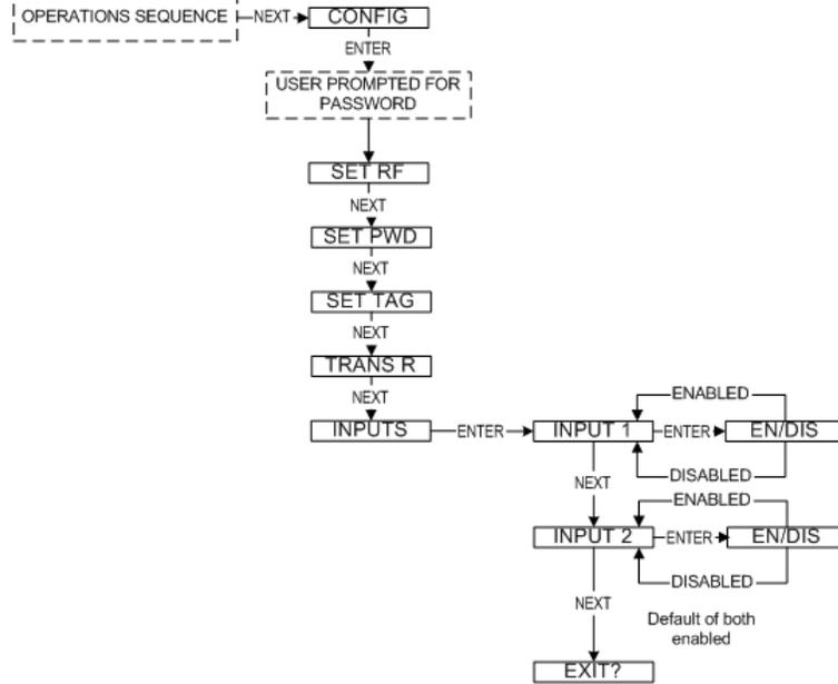
Figure 3-8: Menu Map to Enable the Input Switches
