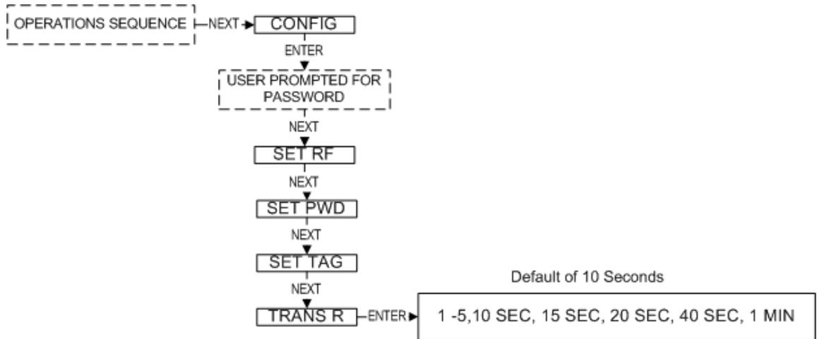
Figure 6-1: Menu Map to the Transmit Rate Setting
