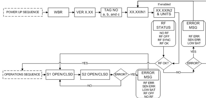
Figure 4-1: Transmitter Power-Up and Operations LCD Sequences
