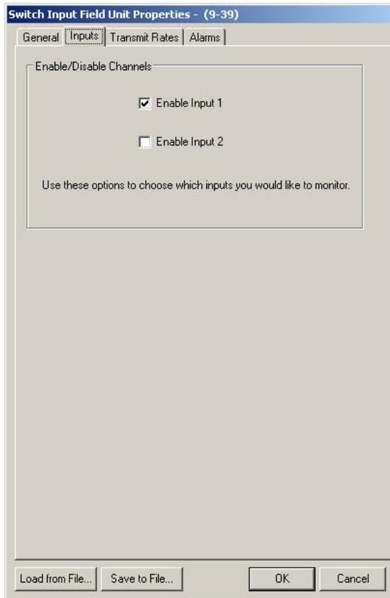
Figure 3-9: Input Switch Configuration using WMT
