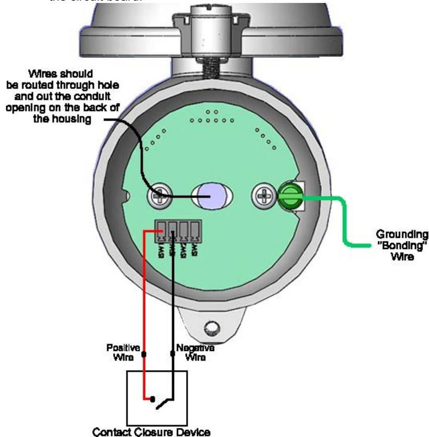
Figure 3-7: Input Switch Wiring Diagram
