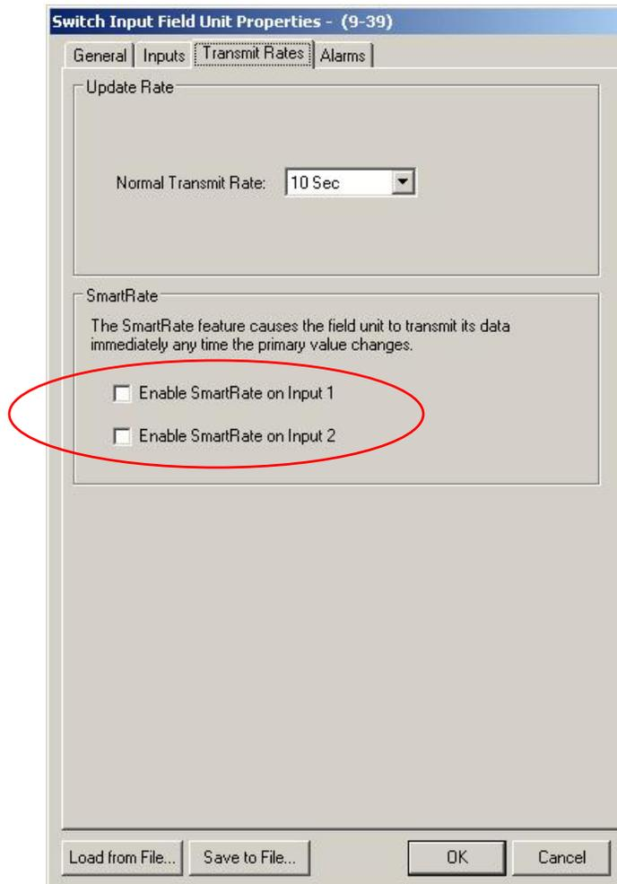
Figure 6-3: Smart Rate Configuration Using WMT
