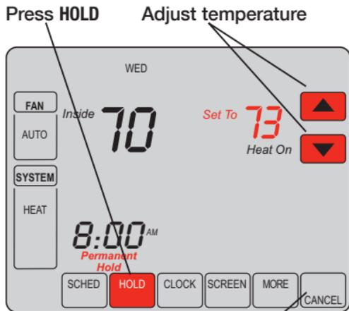
Press **HOLD** to permanently adjust the temperature. This will turn off the program schedule.
