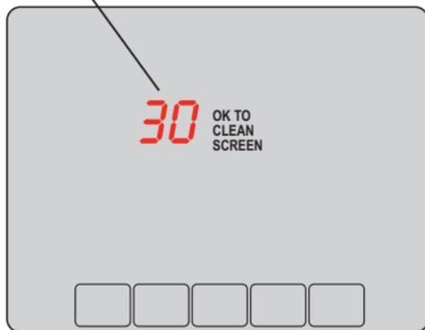
Press **SCREEN** to lock the screen for cleaning. The screen will remain locked for 30 seconds so you can clean the screen without changing any settings.
