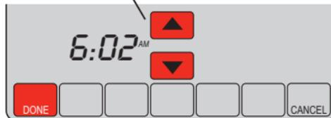
To set the current time display, press **CLOCK**, then press ▲ or ▼ to adjust the time. Press and hold ▲ or ▼ to advance the time more quickly.
