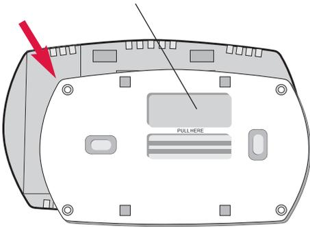
Remove the wallplate from the thermostat as shown at left, then follow directions below for mounting.
