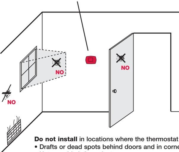
**Do not install** in locations where the thermostat can be affected by:
