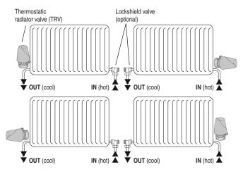
The TRV can be installed on either side of the radiator, in a vertical or horizontal position, as shown at left.
