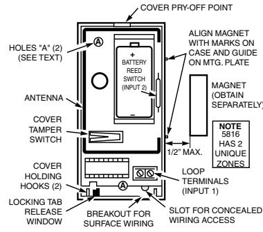
Diagram 2. Transmitter, Cover Removed
