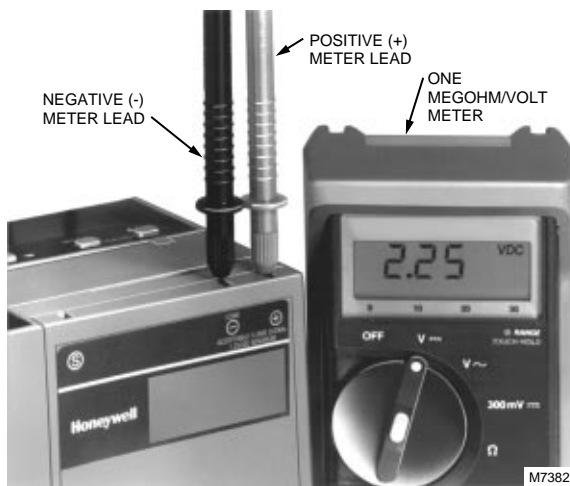
Fig. 18. Flame signal measurement.
