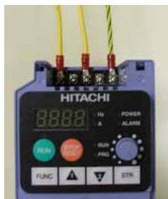
Input wiring for single-phase input (-SFEF and -NFU models)
