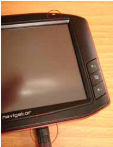
Plug the end of AC adapter or DC charger into the charging connector of GV-590. The power LED will light. When battery is fully charged, the LED becomes green.
