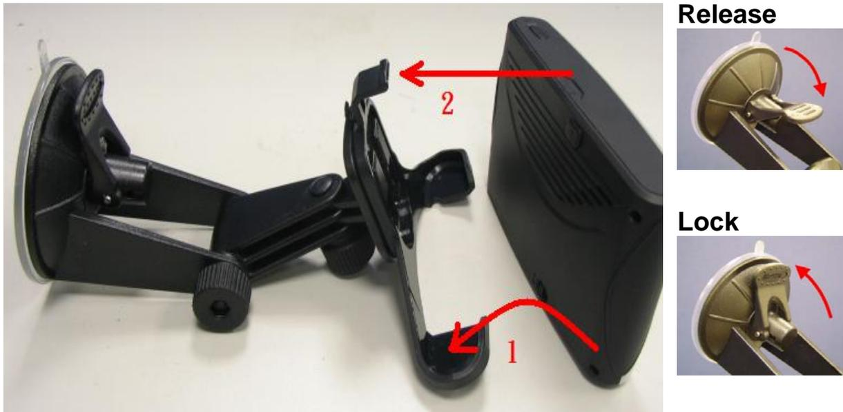
1. Place the GV-560 at a downward angle into the base of the cradle.
