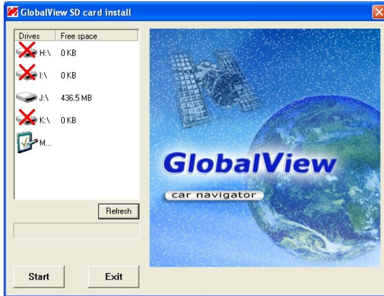
Click on the drive letter which your SD card is inserted, and click on “**Start**” button. After the download process is finished, please remove the SD card from card reader, insert it into your GV-560 and restart it.
