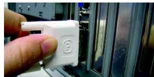
Connect a flat panel display
