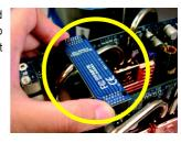
Step 3: In order to securely fix the bridge connector beween the two cards, you must install the retention bracket included with the motherboard and secure the retention bracket to the chassis back panel with a screw.
