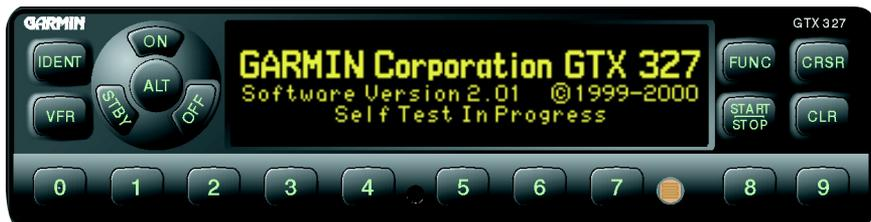
The GTX 327 transponder is powered on by pressing the **STBY**, **ALT** or **ON** keys, or by a remote avionics master switch (if applicable). After power on a start-up page will be displayed while the unit performs a self test.
