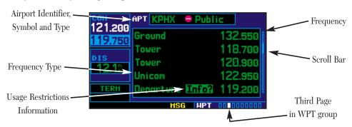
The *airport frequency page* displays radio frequencies and frequency types for the selected airport, as well as sector and altitude restrictions (where applicable). If the selected airport has an ILS approach, the localizer frequency(s) is also listed on the *airport frequency page*. The *airport frequency page* may be used to quickly select and tune a COM frequency. (VLOC frequency is for reference only.)
