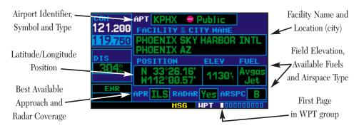
The *airport location page* displays the latitude, longitude, and elevation of the selected airport. The *airport location page* also displays facility name and location, as well as fuel availability, available approaches, radar coverage and airspace type. The following descriptions and abbreviations are used:
