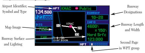
The airport runway page displays runway designations, length, surface type and lighting for the selected airport. The pcl frequency can be transferred to the standby com window by highlighting and pressing to the runway layout and surrounding area is also displayed. The map image scale appears in the lower left corner and is adjustable using the key. For airports with multiple runways, information for each runway is available.
