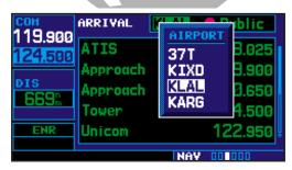
The navigation/communications (NAVCOM) page provides a complete list of airport frequencies at your departure, en route and arrival airports. To place a frequency from this list on standby, highlight the desired frequency and press ENT.
