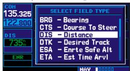
The large right knob  $\textcircled{\textcircled{n}}$  is used to select the data field you wish to change. Then use the small right knob  $\textcircled{\textcircled{n}}$  to display a list of data options and select the desired data item.
