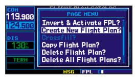
To create a new flight plan, select "Create New Flight Plan?" from the flight plan catalog options.
