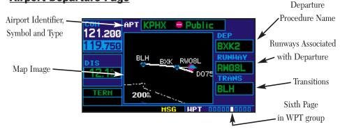
The *airport departure page* shows the available Airport Standard Instrument Departure (SID) procedures for the selected airport. Where multiple runways or transitions are associated with the departure procedure, that information may also be displayed. A map image provides a layout diagram for each departure, runway and transition.
