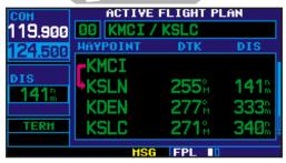
Active flight plan page with flight plan currently in use.
