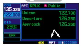
The bottom right corner of the screen indicates which page group is currently being displayed (e.g., NAV or WPT), the number of screens available within that group (indicated by square icons) and the placement of the current screen within that group (indicated by a highlighted square icon). To select a different page within the group, rotate the small right knob ( ).
