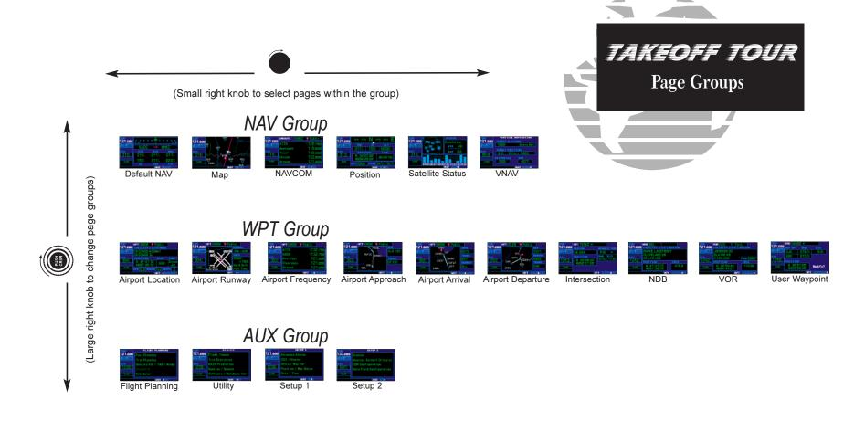
Selection of any main page is performed using the large  $\textcircled{\textcircled{n}}$  and small n right knobs. The large right knob n selects the page group: NAV, WPT, or AUX. The small right knob n selects the desired page within a group. To quickly select the default NAV page, press and hold n.
