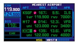
To scroll through the list, press the small right knob ( ), then rotate the large right knob ( ).
