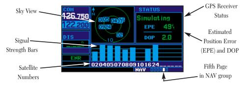
As the GPS receiver locks onto satellites, a signal strength bar will appear for each satellite in view, with the appropriate satellite number (01-32) underneath each bar. The progress of satellite acquisition is shown in three stages:
