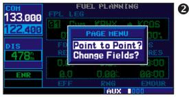
The "Change Fields?" option above is only available on GNC 420 installations which include a Shadin fuel computer. In these installations, use the "Change Fields?" option to review separate fuel information for left and right engines.
