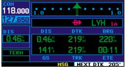
point. 2) A flashing turn advisory ("TURN TO ###") will appear in the lower right corner of the screen when you are to begin the turn. Set the HSI to the next DTK value and begin the turn. 3) The To/From indicator on the HSI (or CDI) will flip momentarily to indicate that you have crossed the midpoint of the turn. For more information on waypoint alerts and turn advisories, see section 5.
