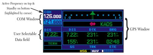
To select the active frequency, you must first enter the frequency in the standby field, and use the key to move it to the active field.
