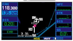
Tuning cursor in the COM window. Use the small  $(\bullet)$  and large  $(\bullet)$  left knobs to dial in the desired standby frequency.
