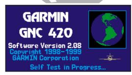
The welcome page appears when the GNC 420 is turned on. During the time this screen is displayed, the GNC 420 performs a self test to ensure proper operation.
