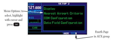
The setup 2 page provides access (via "menu options") to display adjustments, parameters which define the nearest airport search, and COM transceiver channel spacing. When a menu option is selected, the corresponding page will appear providing access to the various unit settings.
