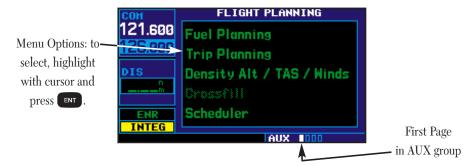
The *flight planning page* provides access (via "menu options") to E6B functions for fuel planning, trip planning, density altitude/true airspeed/winds aloft calculations and a "Crossfill" function to transfer flight plans/user waypoints to a second 400/420/430 unit. When a menu option is selected, the corresponding page will appear providing additional information and features.
