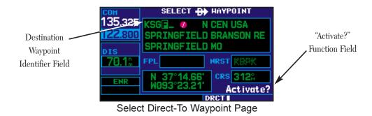
The GNC 420 can use direct point-to-point navigation to guide you from takeoff to touchdown, even in the IFR environment. Once a destination is selected, the unit will provide speed, course and distance data based upon a direct course from your present position to your destination. A destination can be selected from any page with the (direct-to) key.
