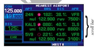
Whenever the GNC 420 is displaying a list of information that is too long for the display screen, a scroll bar will appear along the right-hand side of the display. The scroll bar graphically indicates the number of additional items available within the selected category.
