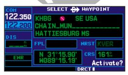
To select the direct-to destination by facility name (shown above) or city location (shown below), highlight the second or third line on the direct-to waypoint page. Use the small ( ) and large ( ) right knobs to enter the facility name or city. The identifier(s) for any matching entries will appear on the top line of the page.
