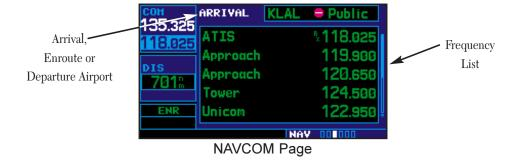
A frequency listed on the *NAVCOM page* can be quickly transferred to the standby field of the COM window. (NAV frequencies are shown for reference only.) This time saving process prevents having to "re-enter" a frequency already displayed elsewhere on the screen.
