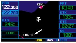
The CLP key allows you to quickly declutter the map display, providing four levels of map detail. Note the "-1" and "-2" ("-3" is also provided) suffix designations above, indicating each successive declutter level.
