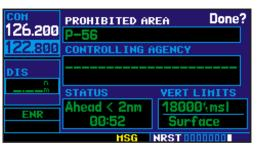
The *airspace page* displays (and airspace alert messages are provided for) the following airspace types:
