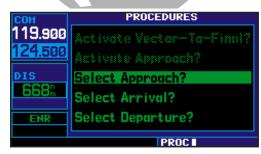
Press the PROC key to display the procedures page. Rotate the large right knob ( ) to select the desired option.
