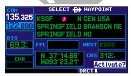
Confirm the selected direct-to destination by highlighting "Activate?" and pressing [EN].
