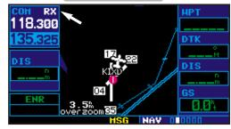
Press the ● knob momentarily to override the automatic squelch. Note the "RX" receive indication when receiving a station.
