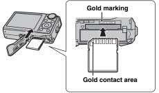
Align the gold marking with the gold contact area, then insert an SD Memory Card completely.
