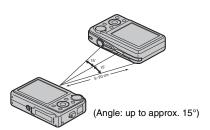
③ Point the camera's infrared port towards the front of the camera's infrared port (→p.11). Transmission distance is about 5 to 20 cm (2 to 7.9 in.) within approx. 15°.
