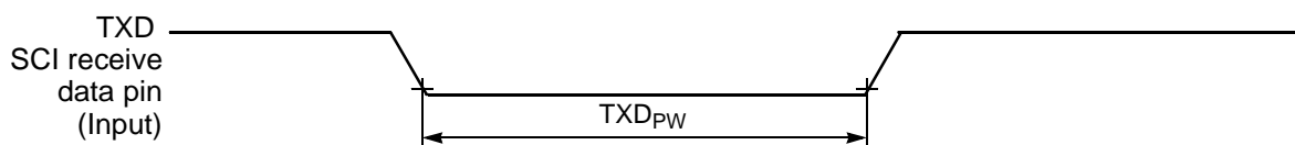
Figure 10-17 TXD Pulse Width
