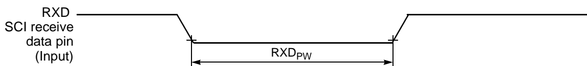
Figure 10-16 RXD Pulse Width
