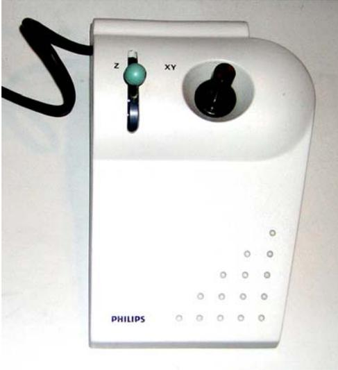
20. Press **A-WOBLER** in **COMPUSTAGE** page (this will initiate back and forth tilting of the goniometer to +/- 15°). Using **Z** control on the joystick, align Z-High by minimizing the apparent movement of the centered feature.
