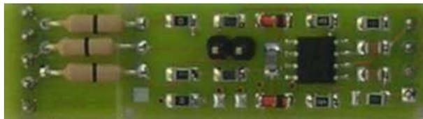
Figure 3.28: The CAN module.
