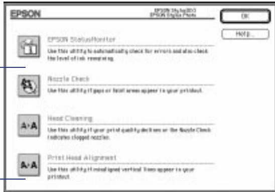
3. Click the Status Monitor icon. The software checks the amount of ink remaining in the printer and displays the Status Monitor window:
