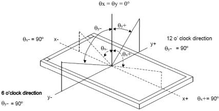
6.2 THE TEST METHOD OF BRIGHTNESS AND UNIFORMITY
