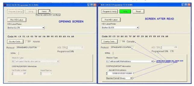
On the screen click on the "Beacon Type" down icon and the three type of programming appear. Select the type programming you wish to use by placing the cursor over the type of programming and click to select.
