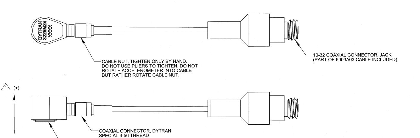
3. CASE AND CONNECTOR MATERIAL: TITANIUM.
