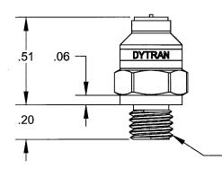
1/4-28 UNF-2A FOR 3086A1 THRU A6 10-32 UNF-2A FOR 3086A1T THRU A6T
