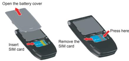
1. Open the battery cover: Hold the phone in one hand, front side facing down and place in middle of palm. Slide the battery cover in the direction as indicated in the illustration.
