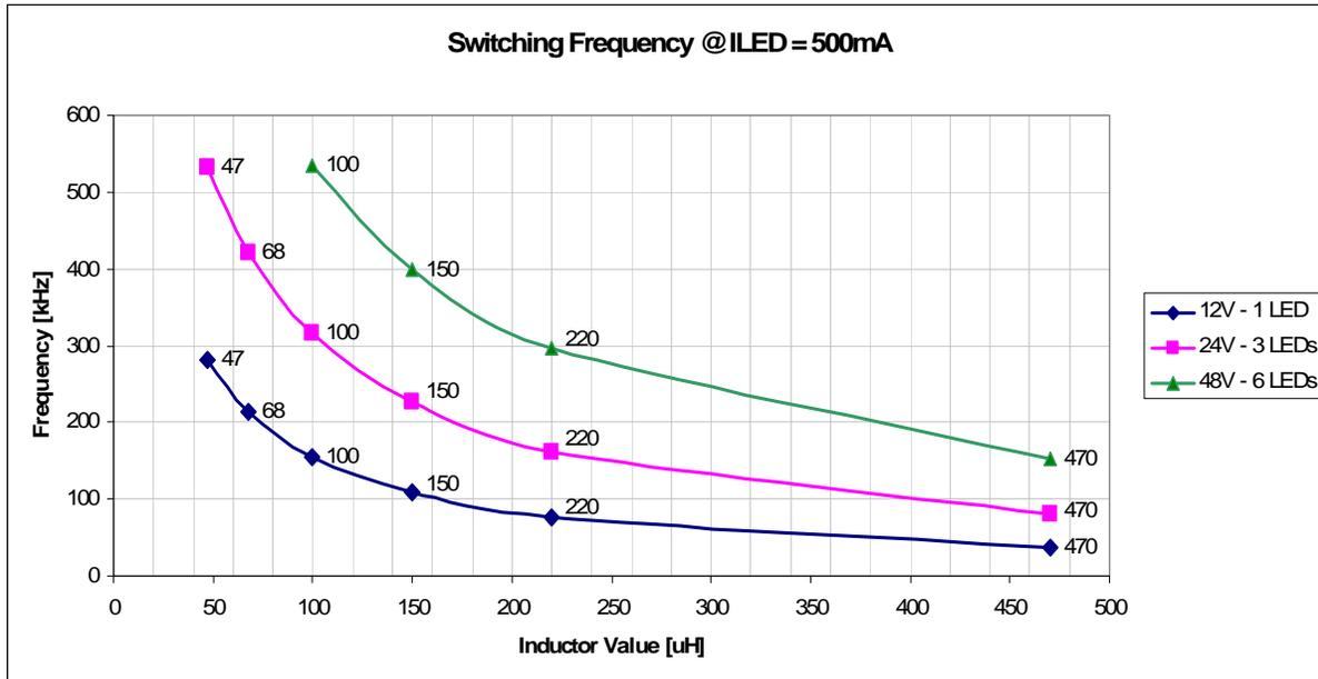
**Figure 4: Switching Frequency Vs Inductor Value**
