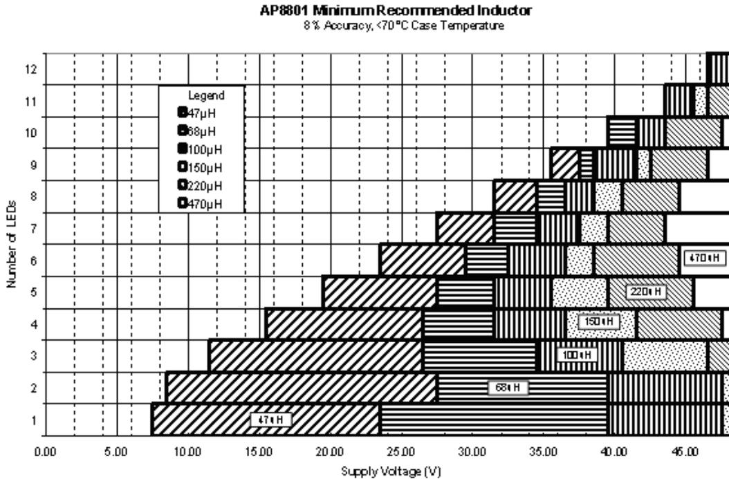
**Figure 5: Minimum recommended inductor with 500mA LED current**
