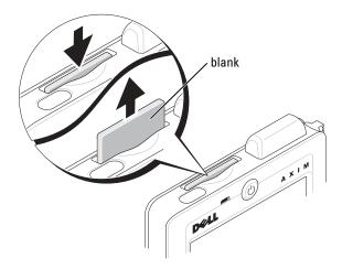
2 Ensure that the card is oriented correctly, and slide it into the slot until you feel a click.
