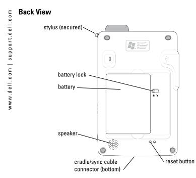
**BATTERY LOCK**—Use this switch to release and remove the main battery. See "Installing and Removing the Battery" on page 23.
