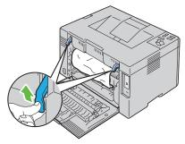
Remove any paper jammed from the back of the printer.
