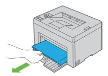
**2** Remove any paper jammed from the front of the printer.
