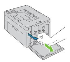
**6** Insert the cleaning rod fully into the hole beside the arrow on the printer until its tip reaches the interior of the printer as illustrated below, and then pull it out.
