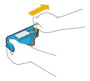
**3** Adjust the toner cartridge to the associated cartridge holder, and then insert it firmly by pressing near the center of the label until the cartridge clicks.
