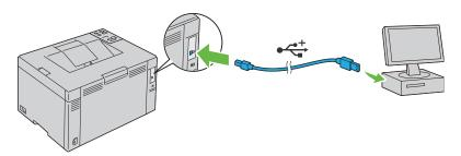
**3** Connect the other end of the cable into a USB port of the computer.
