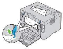
**3** Remove any paper jammed from the back of the printer. If no paper is found in the paper path, then remove any paper jammed out of the output tray.
