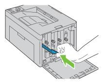
**9** Replace the black cartridge by adjusting it to the associated cartridge holder, and then insert it firmly by pressing near the center of the label until the cartridge clicks.
