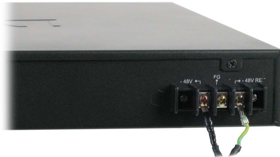
Figure 2 - 4. Power connections attached to contacts on assembly
