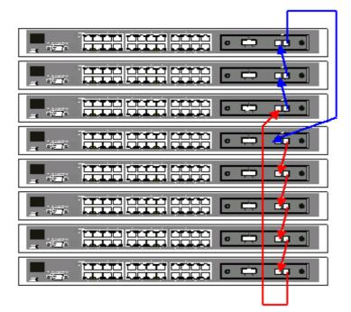
Figure 4 - 2. Switch Stack connections between optional stacking modules
