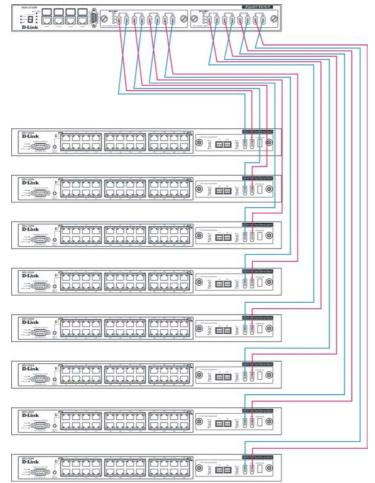
Figure 5 - 1. DES-3226S Switches with DGS-3212SR
