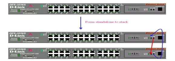
Both Switches are now powered off. Switch B is placed securely in the rack and connected to Switch A via the stacking ports. Both devices are powered on; they recognize the stacking connection and begin negotiating the stacking relationship. Switch A is configured to function as the master device. Switch B automatically assume slave status. Switch A will keep its IP settings and its other configurations remain unchanged. The stack may now be configured as a single entity.
