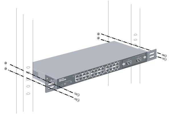
Figure 2-3. Installing the Switch on an equipment rack
