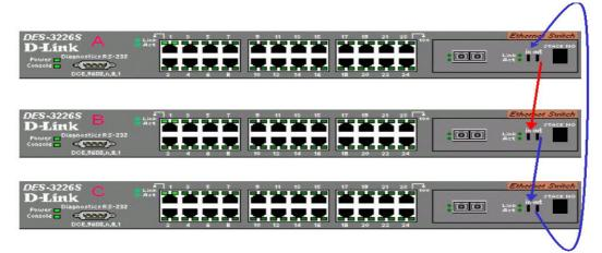
Power on the entire stack. The new stacking arrangement is recognized and the new relationship is negotiated. Switch A retains status as the master of the stack, Switch C is in auto mode and therefore functions as a slave. The stack is ready for operation.
