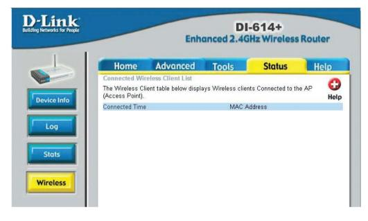
The wireless client table displays a list of current connected wireless clients. This table also displays the time and MAC address of the wireless client connected.
