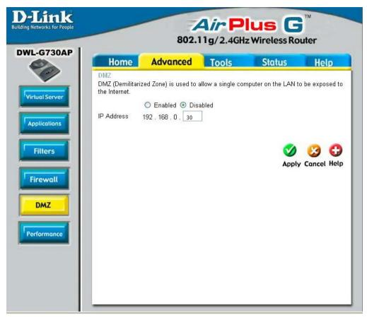
If you have a client PC that cannot run Internet applications properly from behind the DWL-G730AP, then you can set the client up for unrestricted Internet access. Allowing a computer to be exposed to the Internet, this feature is useful for gaming purposes. Enter the IP address of the internal computer that will be the DMZ host. Using the DMZ (Demilitarized Zone) feature may expose your local network to a variety of security risks, so only use this option as a last resort.
