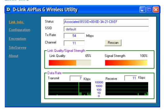
**Status:** Displays the MAC address of the access point that is associated with the DWL-G510.
