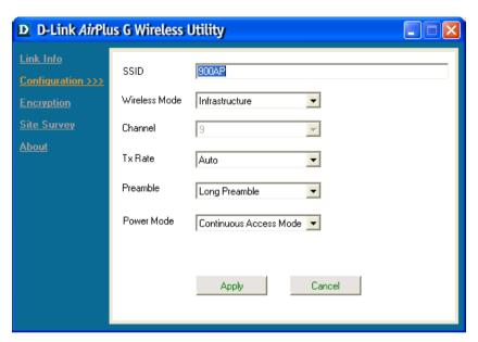
**SSID:** Service Set Identifier is a name that identifies a wireless network. Access points and wireless devices attempting to connect to a specific WLAN (Wireless Local Area Network) must use the same SSID. The default setting is **default**.
