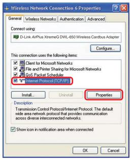
In the window below, select **Use the following IP address**. Input your **IP address and subnet mask**. (The IP addresses on your network must be within the same range. For example, if one computer has an IP address of 192.168.0.2, the other computers should have IP addresses that are sequential, like 192.168.0.3 and 192.168.0.4. The subnet mask must be the same for all the computers on the network.)
