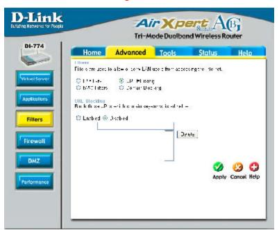
URL Blocking is used to deny LAN computers from accessing specific web sites by its URL. A URL is a specially formatted text string that defines a location on the Internet. If any part of the URL contains the blocked word, the site will not be accessible and the web page will not display.
