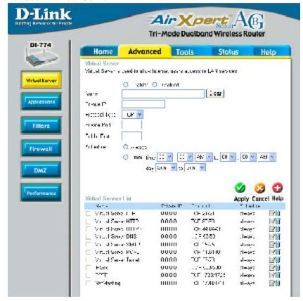
The DI-774 can be configured as a virtual server so that remote users accessing Web or FTP services via the public IP address can be automatically redirected to local servers in the LAN (Local Area Network).
