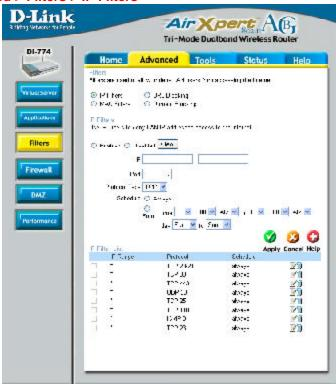
Filters are used to deny or allow LAN (Local Area Network) computers from accessing the Internet. The DI-774 can be setup to deny internal computers by their IP or MAC addresses. The DI-774 can also block users from accessing restricted web sites.
