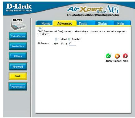
If you have a client PC that cannot run Internet applications properly from behind the DI-774, then you can set the client up to unrestricted Internet access. It allows a computer to be exposed to the Internet. This feature is useful for gaming purposes. Enter the IP address of the internal computer that will be the DMZ host. Adding a client to the DMZ (Demilitarized Zone) may expose your local network to a variety of security risks, so only use this option as a last resort.
