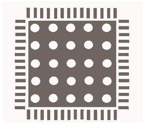
**Figure 16-2a. Plot of the Solder Mask (White Area)**
