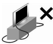
Prevent the power cord from being pressed or kinked by a foreign object. Do not bundle or roll up the power cord to avoid dissipation interruption. Keep your Multimedia LCD Display away from any place where the power cord is easily scuffed. Use only the correct power cord.
