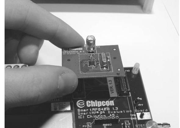
Insert a CC1100EM into both SmartRF04EBs. The connectors will only fit in one position, so that the EM cannot be inserted the wrong way. Do not force the EM. The accompanying PER test requires two-way communication and cannot be run using a CC1150EM.
