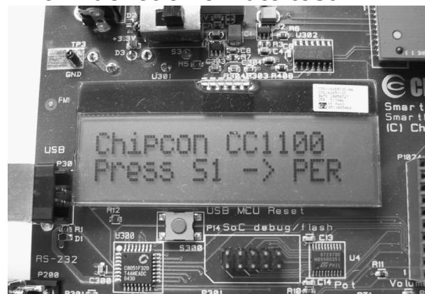
When power is applied to the board, the PER test program will start. You should see the text shown above on the LCD display on both EBs. Press the S1 button.
