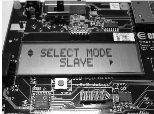
Perform steps 3 through 7 on the second EB. Push the joystick down until you get the display shown above. Leave this EB in slave mode.
