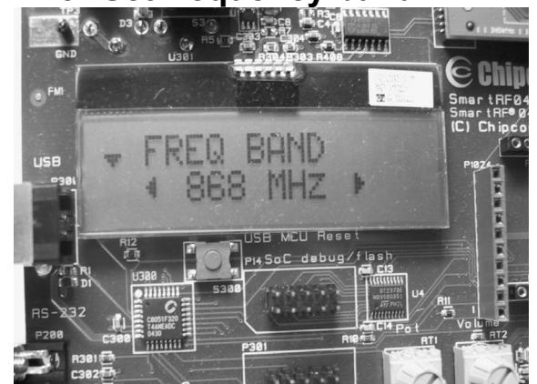
Select the correct frequency band of operation by using the joystick (correct screen shown above for 868MHz operation).
